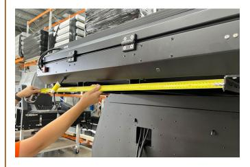
1. Measure and record the distance between the inside vertical faces of the mounting backets on the bottom of the Boss RT1 Roof Top Tent (Item P1).
