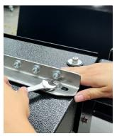
9. Slide the bracket so that the end is flush with the front or rear of the canopy and fully tighten the bolts with a 13mm Spanner (Item T3).
