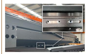
3. Focusing on the <u>Front</u> Canopy Mounting Brackets (Item P2), shuffle the tent so that the very front or rear Hexsert in the brackets aligns with the front of a slot in the tent mounting brackets as shown.
