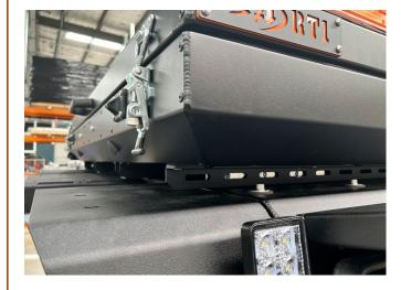
2. Position the tent so that the 2<sup>nd</sup> slot from the rear of the tent mounting brackets roughly aligns with the 1<sup>st</sup> Nutsert in the rear Boss RT1 Tent to Canopy Mounting Brackets (Item P2).
