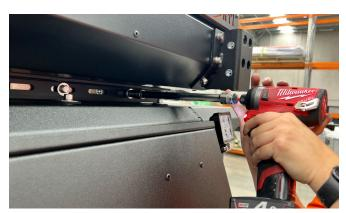
5. With a Power Drive (Item T1), 13mm Socket and 200mm Extension (Item T2), bolt the Tent (Item P1) to the Canopy Mounting Brackets (Item P2) using two (2) M8 x 30mm Hex Bolts (Item F1), M8 Spring Washers (Item F2) and M8 Large Flat Washers (Item F3) per bracket.
