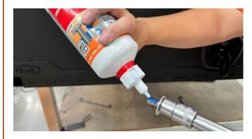
4. Feed one (1) M8 Spring Washer (Item F2) and M8 Large Flat Washer (Item F3) onto eight (8) M8 x 30mm Hex Bolt (Item F1) and cover the thread of the bolts with a generous amount of Loctite.
