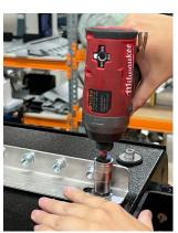
8. Slide the bracket so that the bolt head clears the Hexsert as shown and tighten the bolts as much as possible without locking the bracket in place.
