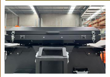
Carefully lift the Boss RT1 Roof Top Tent (Item P1) onto the canopy with the Boss RT1 Tent to Canopy Mounting Brackets (Item P2) positioned between the mounting brackets on the underside of the tent.
