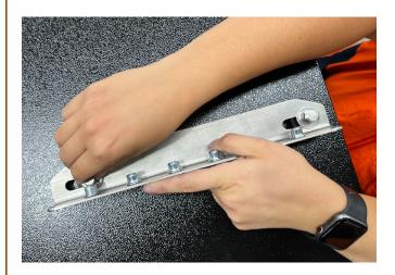
7. Insert the bolts into the Hexserts and tighten by hand.
