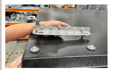
6. Place two (2) Boss RT1 Tent to Canopy Mounting Brackets (Item P2) on one side of the canopy roof and align the bolts with the two (2) Hexserts located at each corner.
