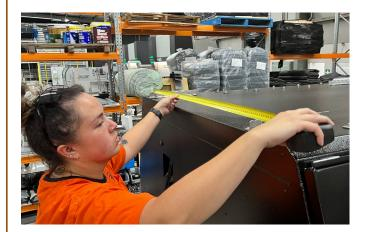
11. Set the width between the outer vertical faces of the Boss RT1 Tent to Canopy Mounting Brackets (Item P2) to **Dim B** recorded in Step 2.
