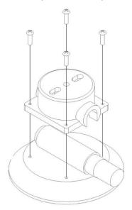
2. Using the Bolt M6 x 30 (6) x QTY 2, Flat Washer M6 x 20 (8) x QTY 2, Flat Washer M6 x 12 (9) x QTY 2, Nylon Lock Nut M6 (10) x QTY 2 and Spacer Plate (11) x QTY 1, bolt the SeaSucker Top (12B) x QTY 1 and Spacer Plate (11) x QTY 1, to Rear Mount Plate (2) x QTY 1. Next bolt the SeaSucker Top (10B) x QTY 2 and Spacer Plate (11) x QTY 2, to Front Mount Plate (3) x QTY 1.
