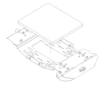
6. Using Bolt M6 x 20 (5) x QTY 4, Spring Washer M6 (7) x QTY 4, Flat Washer M6 x 20 (8) x QTY 4, bolt Side Brackets (1) x QTY 2 to assembled Starlink Mini Cradle (4), making sure the Starlink Mini is held securely in place.
