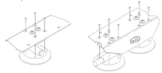
4. Using the Bolt M6 x 20 (5) x QTY 4, Spring Washer M6 (7) x QTY 4, Flat Washer M6 x 20 (8) x QTY 4, bolt the assemblies from step 3 to Starlink Mini Cradle (4) x QTY 1.
