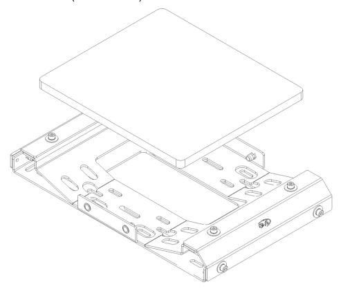
5. Using Bolt M6.0 x 20 (5) x QTY 4, Spring Washer M6 (6) x QTY 4, Flat Washer M6 x 20 (7) x QTY 4, bolt Side Brackets (1) x QTY 2 to Starlink Mini Cradle (4), making sure the Starlink Mini is held securely in place.
