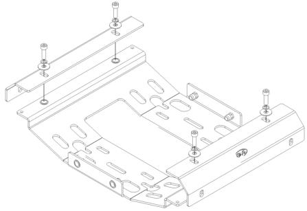
2. Using Bolt M6.0 x 20 (5) x QTY 4, Spring Washer M6 (6) x QTY 4 and Flat Washer M6 x 20 (7) x QTY 4, lower and loosely bolt the assembly from step 1 to the Mounting Base (3) x QTY 1. Once together tighten all 8 bolts.
