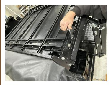
4. Tighten the M8 x 25 Hex Head Bolts (Item F7) on both Awning to Roof Rack Mounting Brackets (Item P3).
