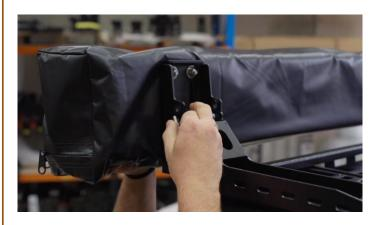
3. Lift the awning onto the vehicle and fasten the Awning Mounting Plate (Item P4) to the front and rear Roof Rack Mounting Brackets (Item P3) with four (4) M8 x 30 Cap Head Bolts (Item F1), M8 Spring Washers (Item F6) and M8 Small Flat Washers (Item F5) per bracket.
