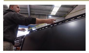
1. Adjust the width between the Awning to Roof Rack Mounting Bracket (Item P3) to match the width between the Awning Mounting Plates (Item P4) on the awning if required.
