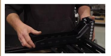
4. Set the Awning to Roof Rack Mounting Bracket (Item P3) over the Unitstrut / Spring Nuts.
