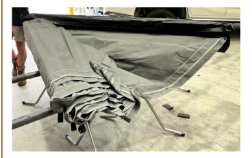
12. With the awning flipped up-side-down, unzip the bag, and partially open the awning to gain access to the Awning Mounting Plate (Item P4) mounting holes.
