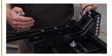
3. Slide the nuts in position along the length of the Unistrut to match the hole pattern of the Awning to Roof Rack Mounting Bracket (Item P3)
