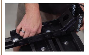
6. Loosely fit a M8 x 25 Hex Head Bolt (Item F7), M8 Spring Washer (Item 2) and M8 Large Flat Washer (Item 5) into the four (4) Spring Nuts
