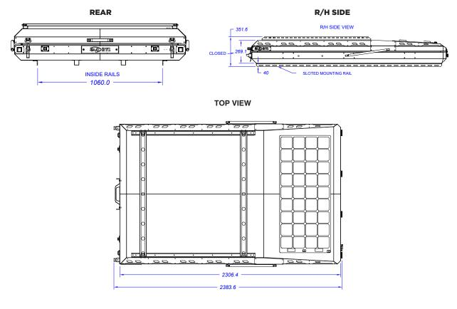
Outside Closed: Inside Open: Weight: Roof Load Limit: 2300L x 1450W x 260W (MM) 2165L x 1315W x 1800H 90 KG Approximately 25 KG
