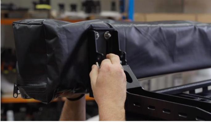
3. Lift the awning onto the vehicle and fasten the Awning Mounting Plate (Item P4) to the front and rear Roof Rack Mounting Brackets (Item P3) with four (4) M8 x 30 Cap Head Bolts (Item F1), M8 Spring Washers (Item F6) and M8 Small Flat Washers (Item F5) per bracket.
