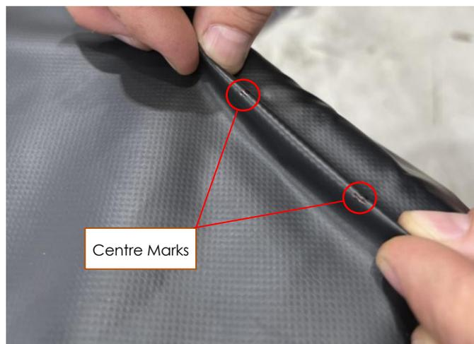
9. Remove the bracket and pinch the bag with the crest crossing through the hole centre marks as shown.
