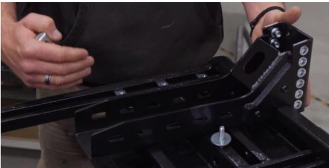
3. Slide the nuts in position along the length of the Unistrut to match the hole pattern of the Awning to Roof Rack Mounting Bracket (Item P3)
