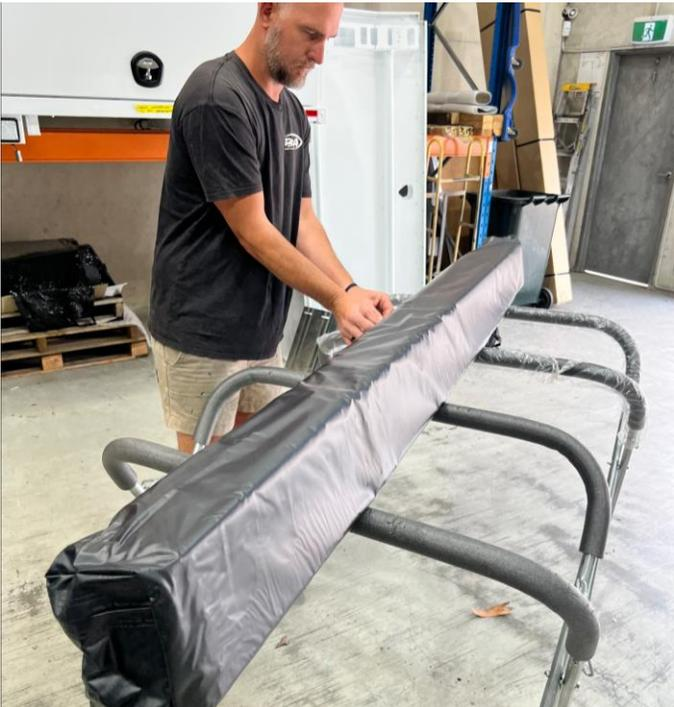
2. Ensure the awning is oriented correctly in the bag, the 'Boss Aluminium' logo must be located at the front end of the awning.
