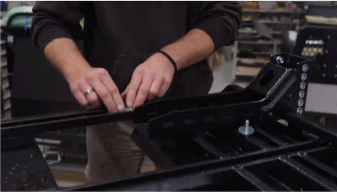
1. Insert four (4) M8 Spring Nuts (Item F8) into the Unistrut rail at the very rear of the Boss Low Profile Roof Rack.
