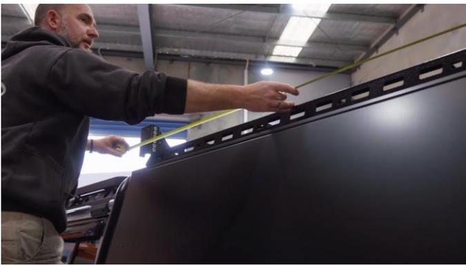
1. Adjust the width between the Awning to Roof Rack Mounting Bracket (Item P3) to match the width between the Awning Mounting Plates (Item P4) on the awning if required.
