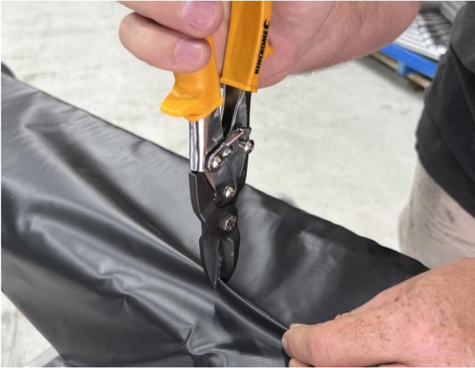
10. At each hole centre mark, cut approximately 5mm down from the crest of the fold to create an 10mm slit in the bag.
