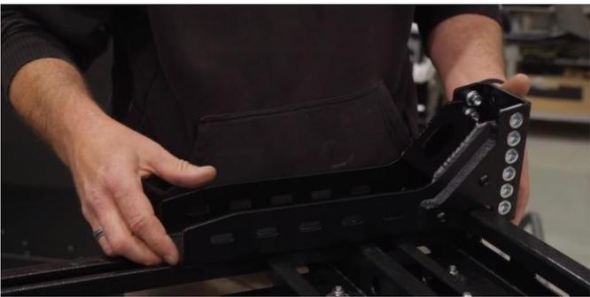
4. Set the Awning to Roof Rack Mounting Bracket (Item P3) over the Unitstrut / Spring Nuts.
