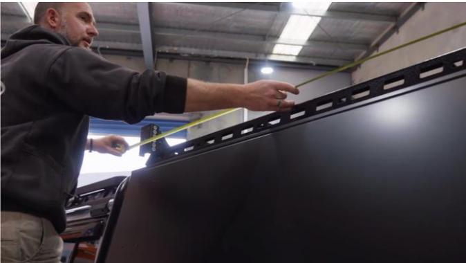
1. Measure and record the centre-to-centre distance between the Awning to Roof Rack Mounting Brackets (Item P3).
