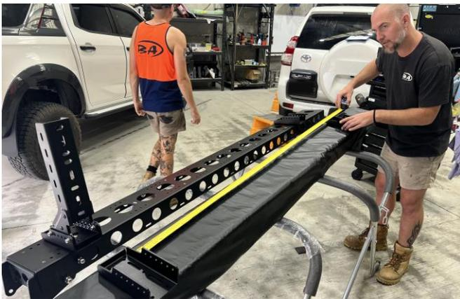
18. Feed four (4) M8 x 25 Hex Head Bolts (Item F3) through the front end of the awning and bag as shown.
