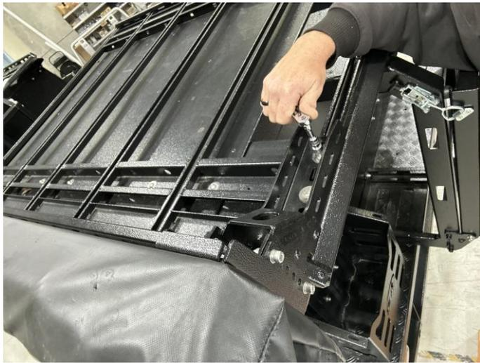
4. Tighten the M8 x 25 Hex Head Bolts (Item F7) on both Awning to Roof Rack Mounting Brackets (Item P3).
