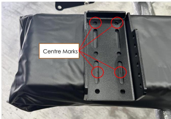
8. With a permanent marker, mark the centres of the two holes and two slots as shown.
