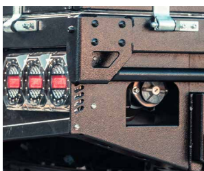
Step Quarter Panels Increase tray strength by bracing the Rear Infill and Under Body Boxes
