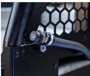
Headboard Fill point for Water Tank
